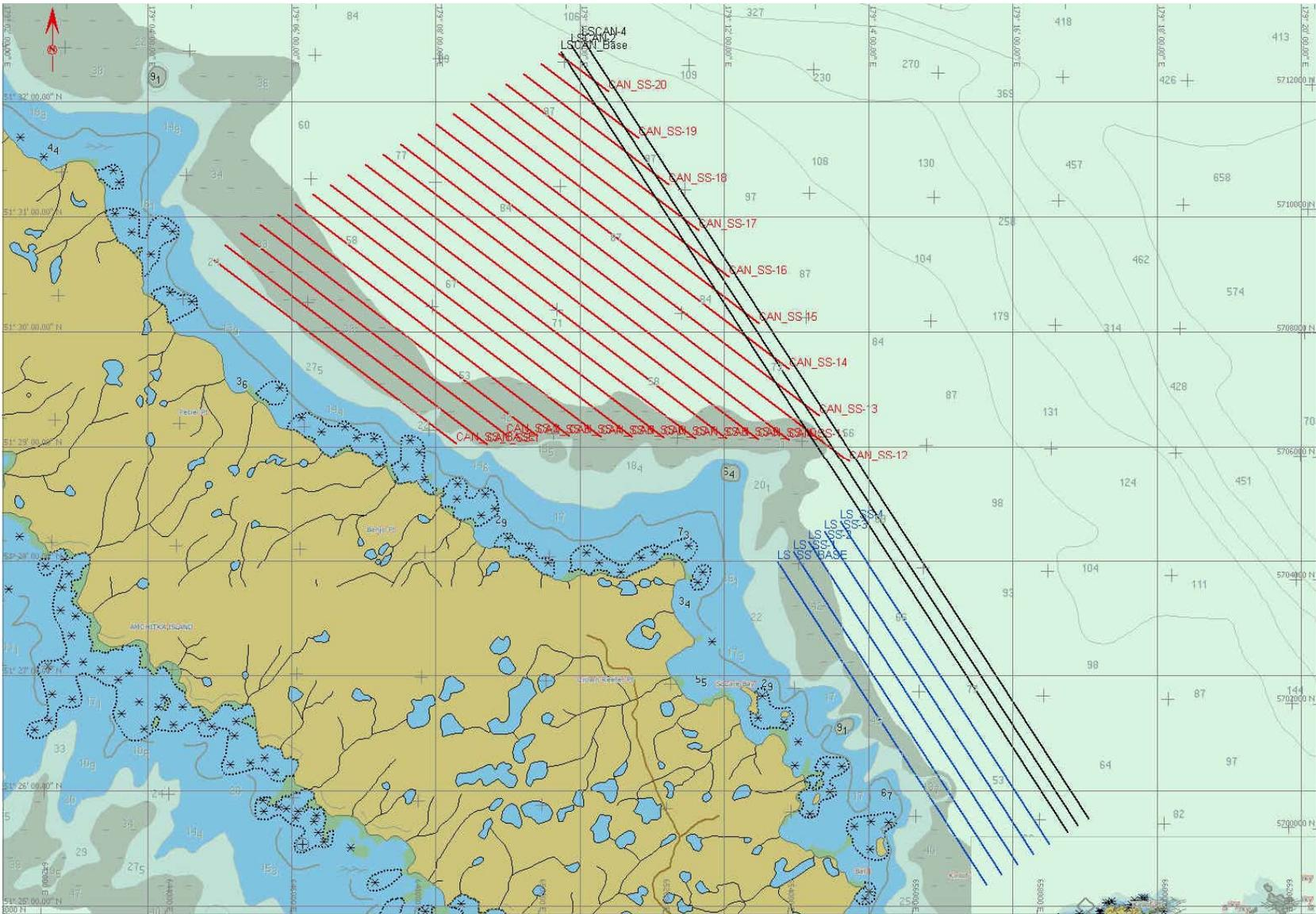
Figure 10. Transect lines for the side scan survey.
