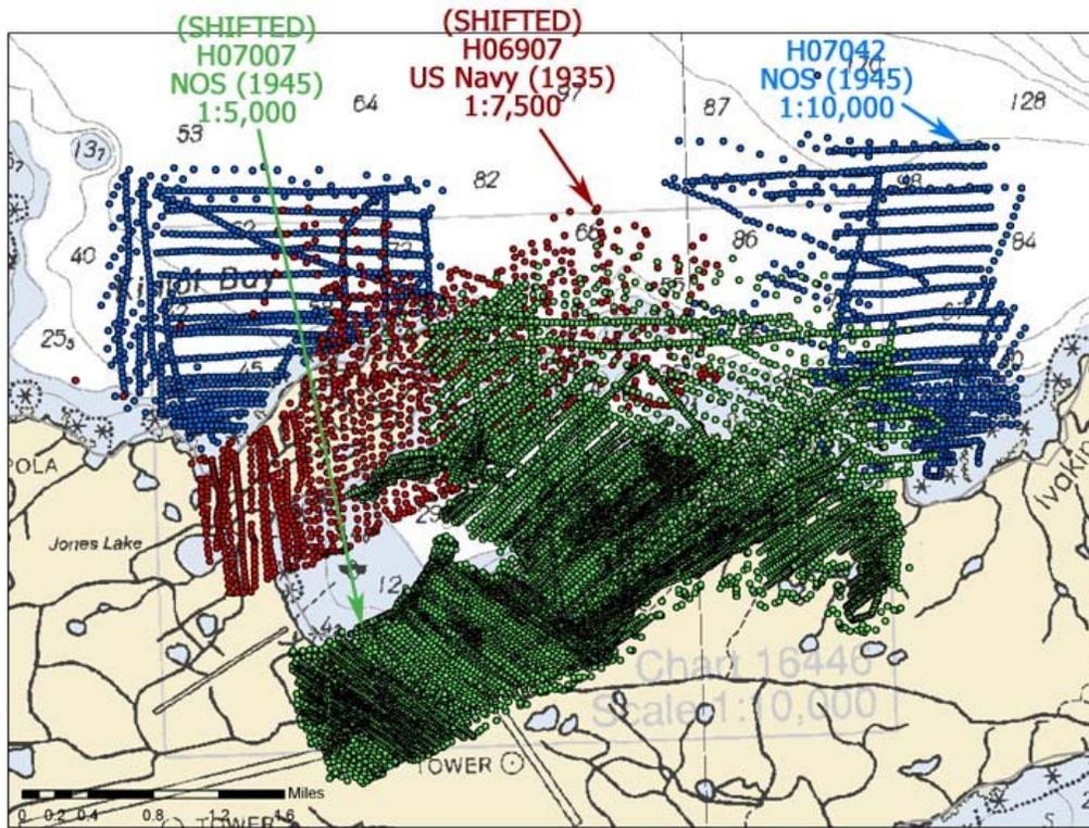
Figure illustrating probable horizontal control problem in two 1935 and 1945 Constantine Harbor surveys.
