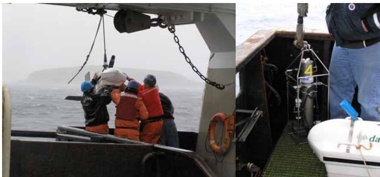
Figure 3.12 Deploying the Sidescan sonar. (Photos D. Volz)
