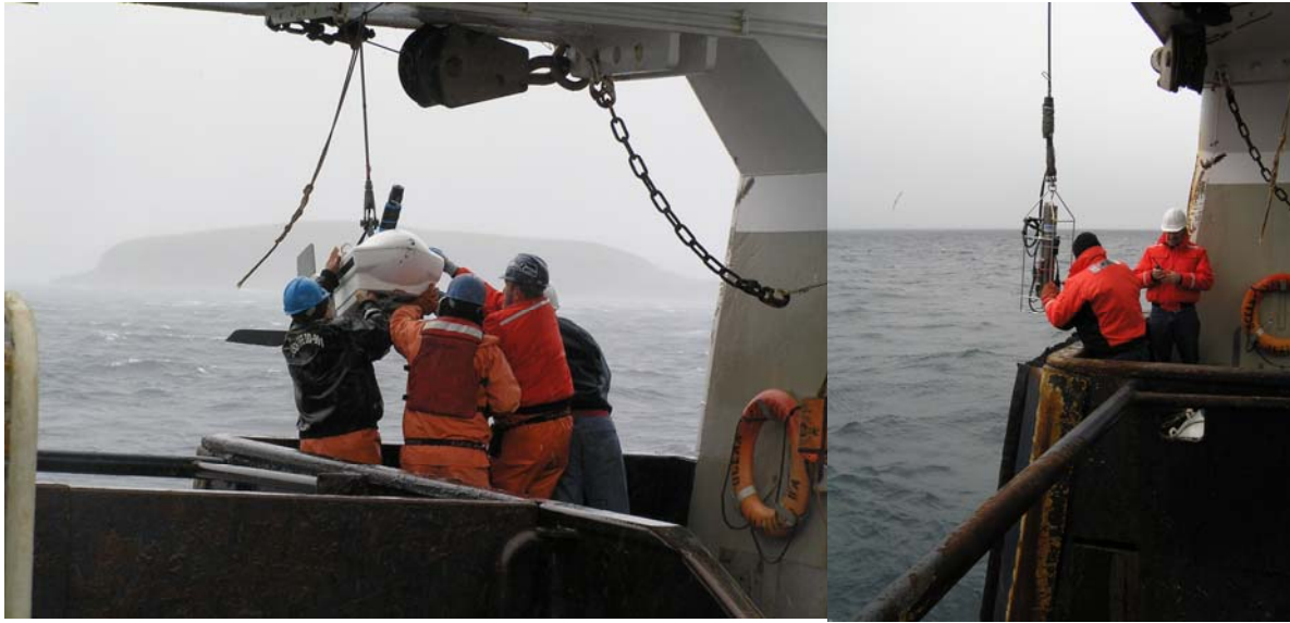
Figure 4.7. Deployment of Side-scan Sonar (Photos D. Volz)
