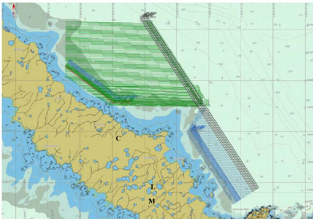
Figure 5.3. Survey lines for bathymetric survey. Approximate locations of test sites are shown.
