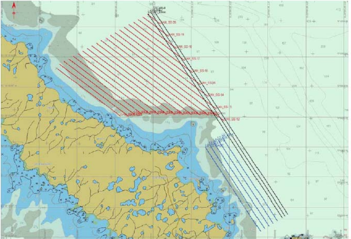
Figure 5.5. Transect lines for the side scan survey. For approximate locations of Cannikin (C), Long Shot (L) and Milrow (M) see Figure 5.3
