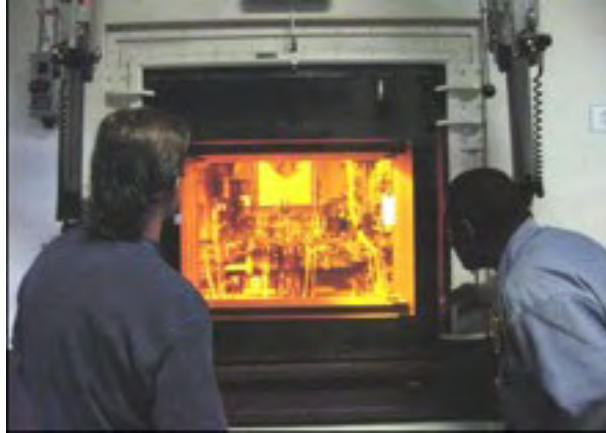
Figure 2. Electrorefiner operational in the hot cells of the Fuel Conditioning Facility
