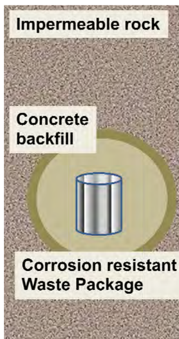
Figure 7. Example of an engineered and natural barrier designed to complement. After a design considered by the European Commission. See: http://itu.jrc.ec.europa.eu/index.php?id=169
