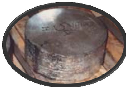
Figure 6. Photograph Compacted Hulls and Hardware Metal Slug (Courtesy of Areva)
