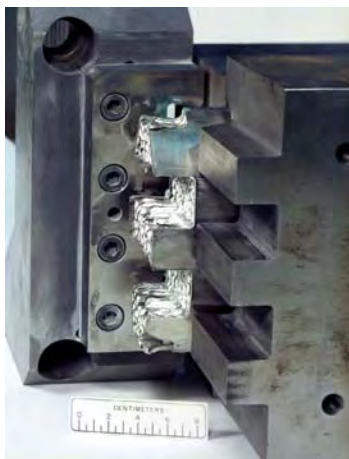
Figure 3. Typical Fuel Shear Blade Design (Croff, 1997).
