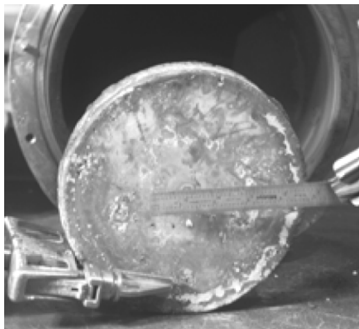
Figure 10. Metal Slug from Electrochemical Processing of EBR-II Fuel (Courtesy of INL)
