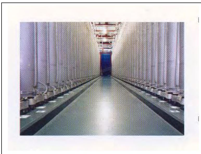
Figure 15. Cascade hall of advanced centrifuges at Urenco's Capenhurst Plant, UK (reference 2).
