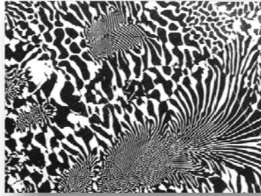
Figure 9. Microsturcture of Fe – 15% Zr Alloy (from Ebert 2005)
