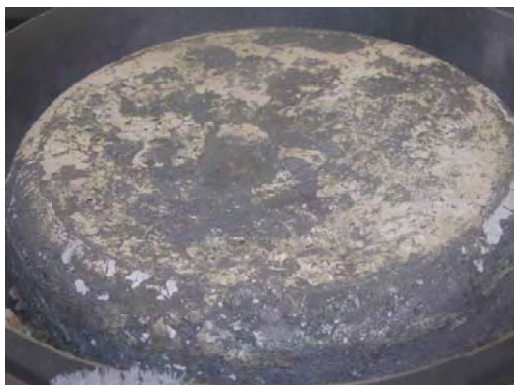
Figure 7. Photograph of Low-temperature (85% SS, 15% Zr) Alloy Slug (Courtesy of INL)
