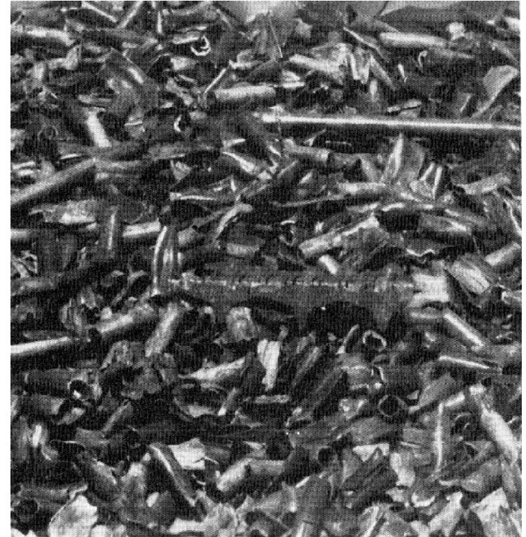
Zircaloy and SS Scrap from Cogema Plant, LaHauge from: Management of Cladding Hulls and Fuel Hardware, Tech report 258, IAEA, Vienna, 1985
