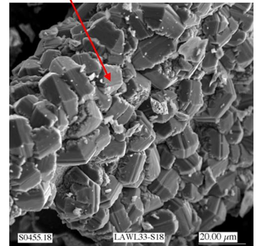
Secondary phase precipitation reaction consumes aqueous components causing more glass to dissolve.
