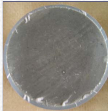
Precipitate on sample AMG-B after 6 th leaching interval
