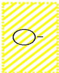
**Area with TRU contamination, moderately controlled, and a regulated above ground storage tank**
