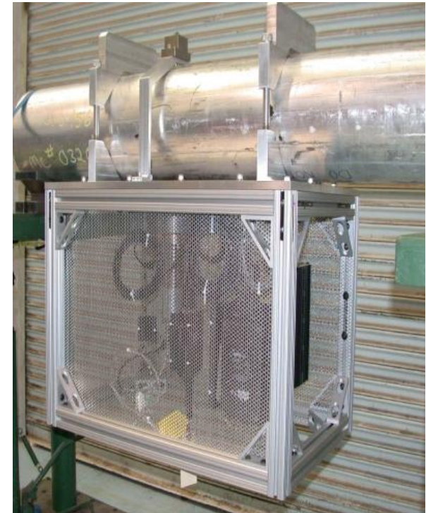
Blend Down Monitoring System equipment placed on the pipes of Russian down blending facilities
